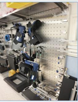
Many accessories that are used for storage and fixation already belong to the **opFIX®** range of products: Hooks of various lengths, standard equipment rails, flat storage, baskets, container for incidentals (stainless steel or plastic) and more. The range of products is being continuously extended. Customer-specific solutions are also possible. Just talk with us.
